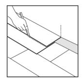
Radiators (or upright construction elements in the area): cut the element to size accordingly. In the case of radiator pipes, add at least 5 mm to the diameter of the radiator pipe.
