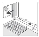
Before installation of the elements, the centre axis of the room must be defined. This depends on the shape of the room and the design of your flooring. Start installation in the centre of the room. Boards are always pressed down from the centre towards the edge. The installation direction is determined according to the installation plan and, if necessary, taking the installation arrows into account.
