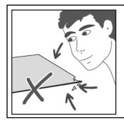
During installation, mix elements from at least three or more packages from the same batch and check them for material faults. Elements with visible material faults must not be installed.
