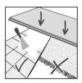
The right preparation of the substrate is key to the successful installation of design flooring 555 too. Roughness or unevenness of the substrate can press through the new floor covering and lead to increased wear at the spots affected. Insufficient preparation can lead to an unsatisfactory appearance or even clear joint formation.
