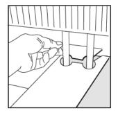
After a period of approx. 30-45 minutes (depending on the room climate conditions), the covering has to be rolled cross-wise using a press-on roller weighing at least 50 kg.
