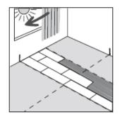
During further installation, apply the adhesive in sections according to the manufacturer's specifications and then join the next elements together exactly by placing the elements in the adhesive bed with light pressure. It is important to install the flooring joint-tight and tension-free. The partial areas should be rolled using a suitable hand roller immediately before further installation.
