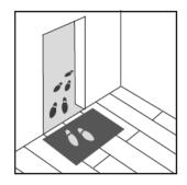
Near French windows and overhead glazing, ensure there is sufficient shade, so that the surface temperature of the floor covering does not exceed the limit of 29°C. In areas where a higher temperature load or increased surface moisture is to be expected, 2-component adhesive should be used.
