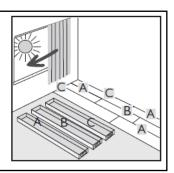
Cut the elements to size as described before and simply place these in the adhesive bed.
