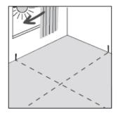
The area to be glued is marked by a chalk line so that the adhesive can be applied after the elements have been removed again. The adhesive manufacturer's specifications must always be heeded. Do not continue until the installation work until the starting rows are fixed permanently. Only use the products approved by us in the adhesive recommendation.
